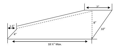
Rear sail panels must be the same left and right, either both open or both closed. The sail panel must drop towards the deck at the back edge of the roof panel. Sail panel maximum length is 45". The sail panels cannot connect to the rear spoiler (see illustration).
